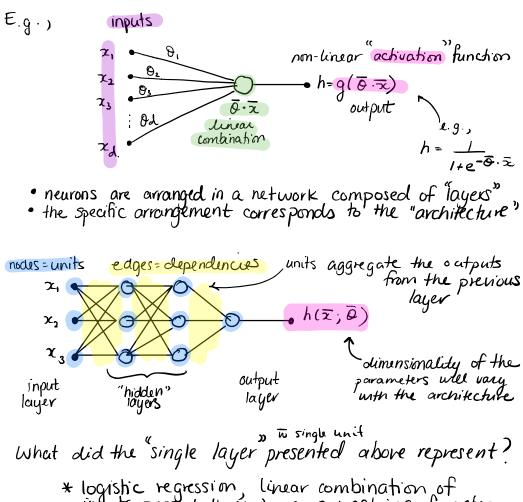
\* logistic regression, linear combination of inputs passed through a squashing function  $\hat{y} = h(\bar{x}; \bar{\sigma})$  $= \frac{1}{1+e^{-\bar{\sigma}\cdot\bar{x}}}$
